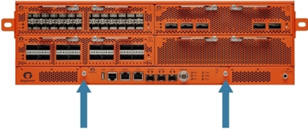
Figure 15: Extension Board Screw Location on GigaVUE-HC3 Front
