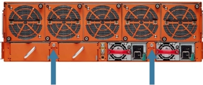
Figure 10: Fan Tray Screw Location on GigaVUE-HC3 Rear
